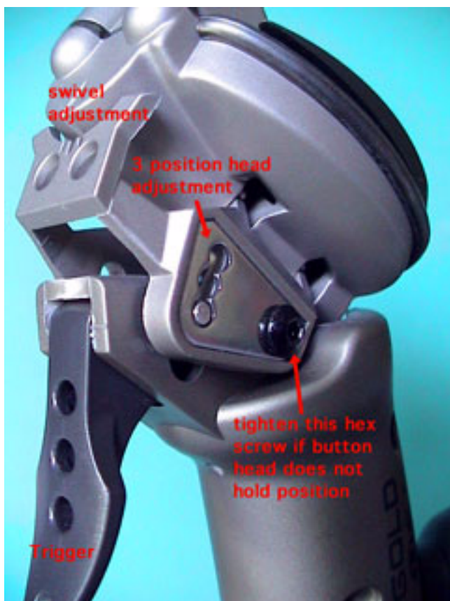
Button head, and the hex screw that may need tightening.
