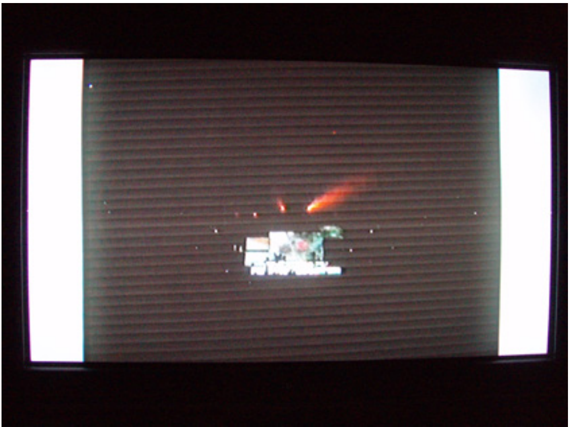
Playing videos from the HomeDock Deluxe result in a picture filled with horizontal bands.
