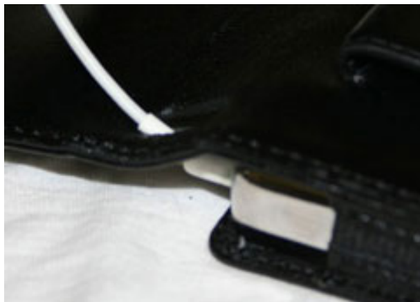
The headphone cutout is fairly small, which puts pressure on the stock Apple earbuds and may prevent the use of headphones with larger plugs entirely.
