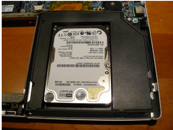
The OptiBay replaces the internal SuperDrive with a hard drive.
