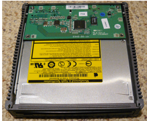
The SuperDrive in its new external enclosure.
