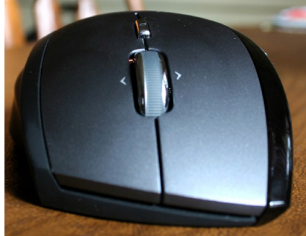
The Revolution's scroll wheel is not clickable, but the button behind it is.
