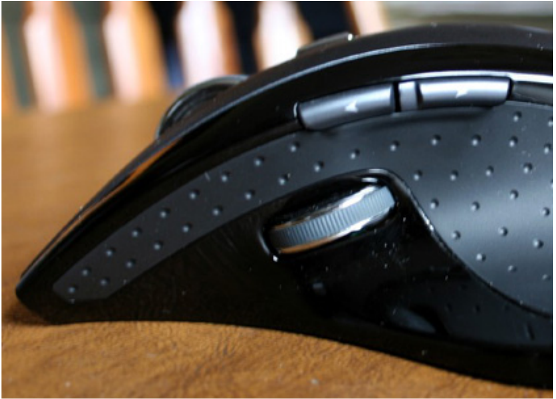
The Revolution includes a thumb “wheel” and two additional buttons on the side.
