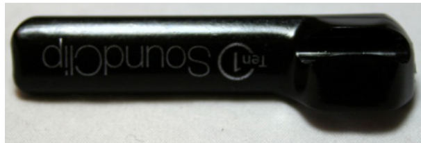
SoundClip (yes, it's upside-down) by itself. Note the cable clip on the right, for retaining SoundClip on the sync cable while docked or charging.
