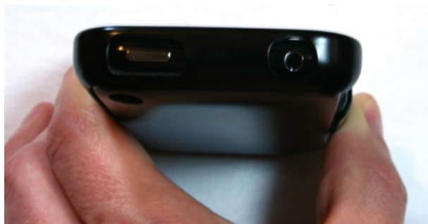
The deep headphone jack cutout is highly protective yet big enough for even the largest headphone plugs.
