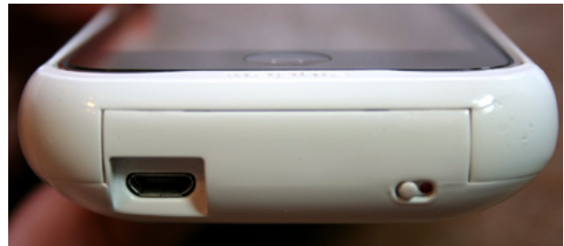
Here’s a close-up of the mini-USB connector and the charging switch. It would have been nice if Mophie could have engineered a Dock Connector pass-through to avoid the extra cable, but they thoughtfully include the appropriate USB cable.
