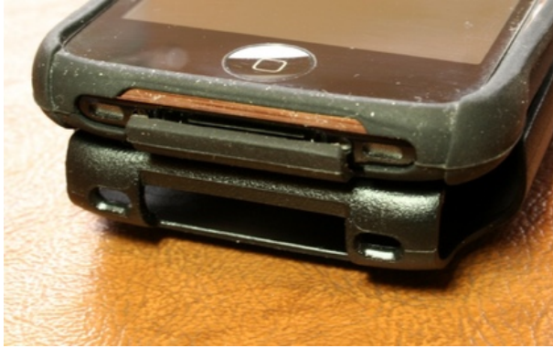
This flexible cover does a great job of keeping gunk out of the dock connector.
