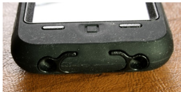
A thick silicone plug protects the dock connector, although the speaker and microphone are (logically, since otherwise it would get awfully quiet) still exposed.
