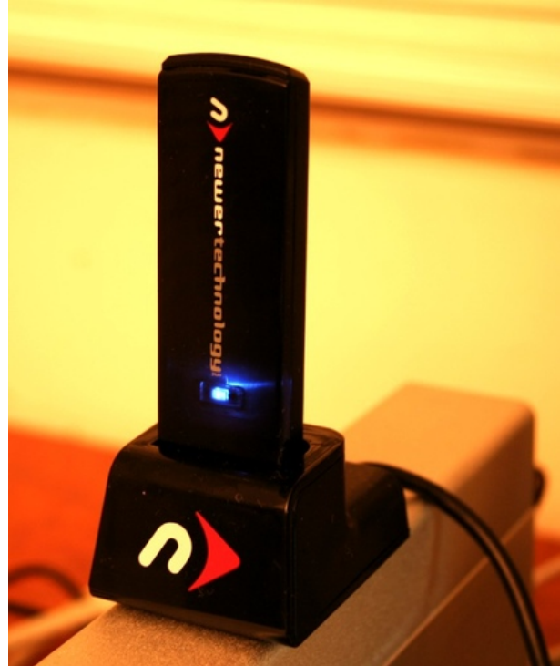
The USB extension cradle allows you to regain use of adjacent USB ports by moving the bulky plug away from your Mac or USB hub. Don't try to sleep in the same room if you like it dark, though—that blue LED is amazingly bright.
