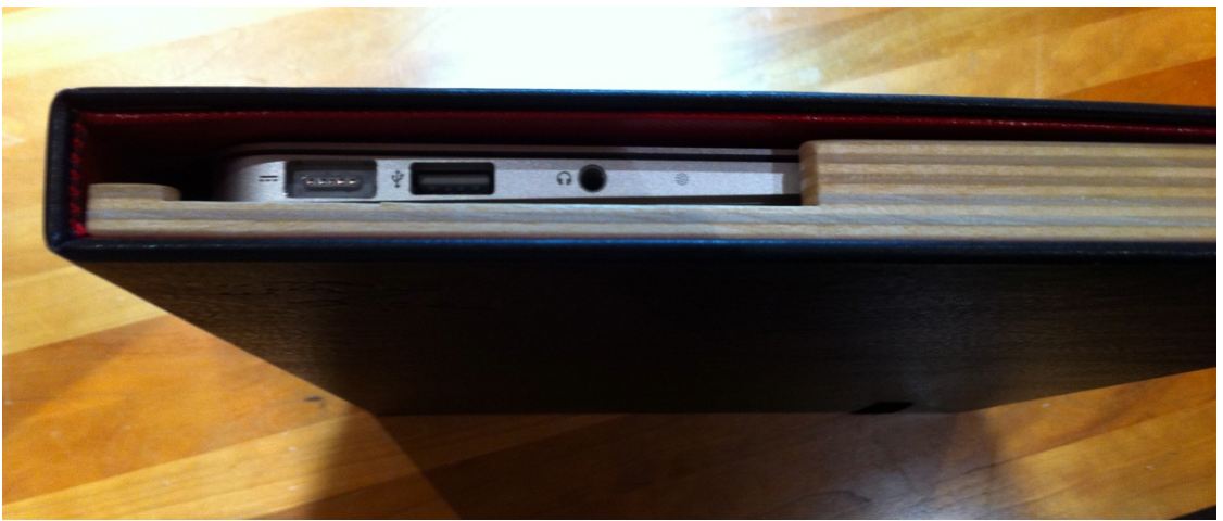
With MacBook Air inside—note slight bowing of front cover.
